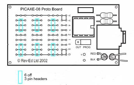
Using the bare wire remaining from the resistors, link the remaining pads as show.
